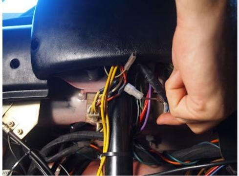
Plug in new AMP connector in between:
