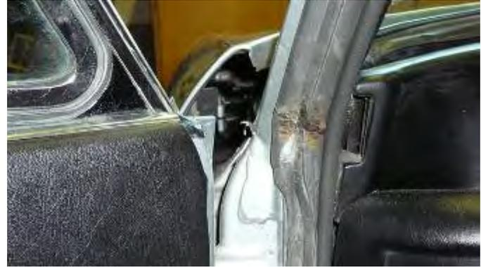
The next step is to position the keepers on the side of the apron. This is accomplished by bringing them outboard and finger tightening both screws. As you close the hood, it will position them in the correct place. Repeat this step and peek with the door open, to make sure they just touch the sides of the stoppers. The keepers can also be used to push the side of the hood outboard in order to make them flush with the side of the door.
