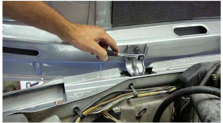
Secure both torsion arms to the apron brackets. Slide the arms all the way to the front. Make sure that your washers are positioned such that the attaching point allows the arm to rotate freely. **CAUTION:** do not ever attempt to close the hood with these loose, make sure they are tight on the apron slides - otherwise, you will end up with some nice scratches on your apron.
