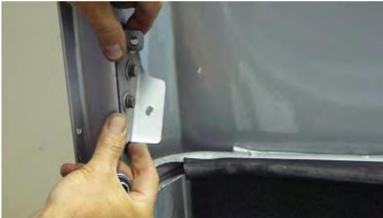
These brackets can slide up and down and back and forth. It is possible to pivot them, but I recommend keeping things simple and restrict the adjustment to straight moves only.
