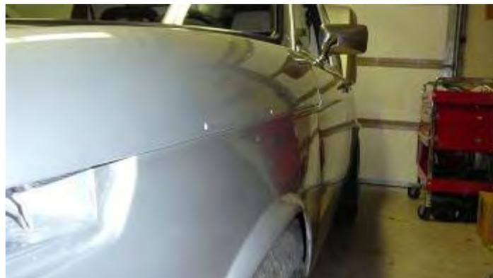
The position of the torsion bar arms on the apron slides controls both, the door gap and the flushness with the doors. Slide them to the back and you will close the door gap. Slide one side more than the other and you will adjust flushness. At this point, what you want to achieve is flushness first, with an adequate gap on at least one side. Play with the slides until you accomplish this.
