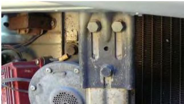
Once the two front hinges are secured to the car, I recommend recruiting two other people to hold the hood and position the hood, while a third person bolts the hinge screws. Push the hood on the hinges as far down, this actually is moving the hood forward at the close position. **DO NOT CLOSE THE HOOD yet!**
