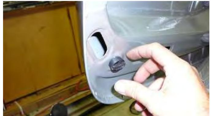
Finally, the two vibration dampeners are installed in the front. These screw in or out for adjustment. These can lift the front corners of the hood slightly and improve the front hood gap.
