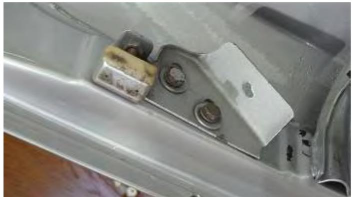
Remove the angle brackets so they will not interfere with the next adjustments.
