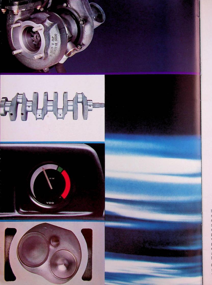
In everyday road usage with normal motoring requirements, full engine performance is ready to be called upon. The turbo-supercharger starts off gently at a low rev. count. The engine, tuned to high performance, runs with little noise. Without vibrating. Without jerking. The exceptional performance of the BMW 2002 turbo requires exceptional design technology: an oil cooler. An exhaust system of highly heat-resistant material.
