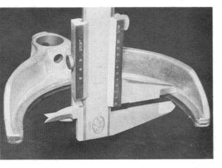
Check selector forks for wear<sup>1</sup>) and renew if necessary.
