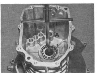
Determine distance A from housing sealing surface to grooved ball bearing, e.g. 150.9 mm (5.941").
