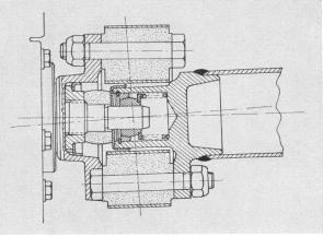
**Fitting instruction:** Do not damage the screw cap. Check free movement of centering bearing and pack with Longterm 2 if necessary.
