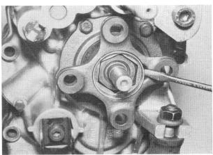
Push guide sleeve 607 onto centering pin. Hold flange with retaining spanner 6039, unscrew flange nut and pull off flange.
