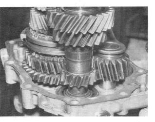
Pull the shift rod with lever and the reverse gear pinion out of the gearbox cover. Note that balls may escape.
