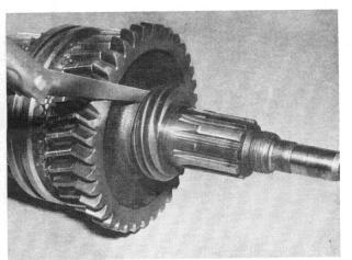
Insert shim Y in front of reverse gear pinion.
