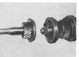
Remove drive shaft, selector sleeve and needle cage. Fitting instruction: Check synchromesh unit; see page 23-00/29.
