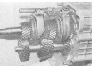
Place selector forks of 2nd/3rd and 4th/5th gear in the selector sleeves.
