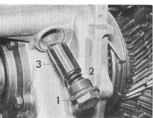
Remove screw plug (1). Take out spring (2) and locking pin (3).
