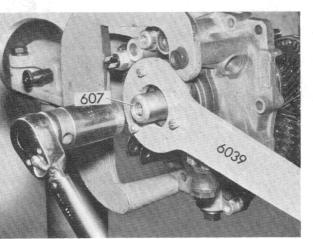
Push selector rod (5) into 2nd gear position. Turn guide sleeve until the locating pin (6) can be driven out properly.
