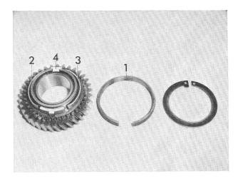
**Note:** The synchromesh ring for first gear is more oval in shape than the rings for second, third and fourth gears.
