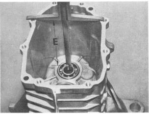
Determine distance E from housing sealing surface to grooved ball bearing, e.g. 150 mm (5.905").
