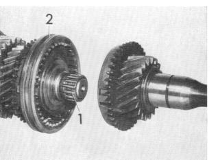
Pull the input shaft with needle roller cage (1) and selector fleeve (2) away from the output shaft.
