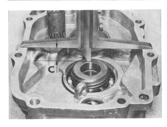
Before fitting gearbox cover, check axial play¹) (B) of the double gear.
