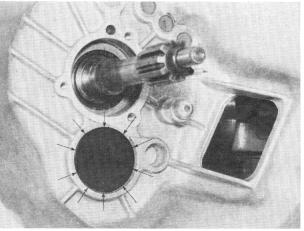
Heat gearbox housing around sealing cover so that the ball bearing on the layshaft slides out easily.
