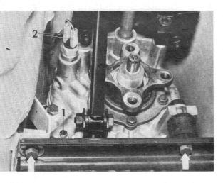
Slacken bolt (1) and pull out speedometer shaft. Pull off cables (2) for reversing light switch. Slacken crossmember.
