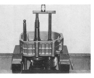
Position an approx. 135 mm (5.25") long tube on the hex. head bolt of the layshaft. Lay a flat bar on the output shaft and tube. Press out gear assembly.
