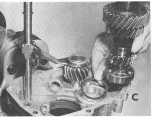
Insert arrestor ball, press downwards and push reverse gear selector rod with reverse idler pinion into housing cover until 1st arrestor locates.
