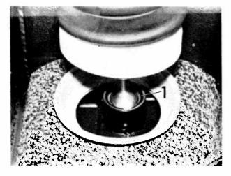
Push up gaiter and foam rubber ring. Lift out circlip (1).
