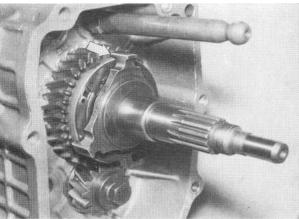
Push 1st gear pinion and guide sleeve onto output shaft.
