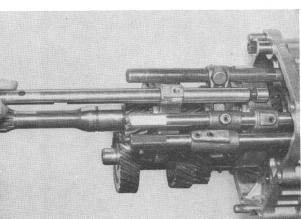
Move shifting sleeve for fourth gear and fifth gear into idling position.
