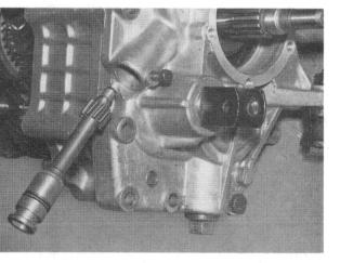
Remove speedometer pinion.
