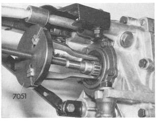
Renew radial sealing ring on output flange.
