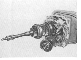
Push drive and output shafts into housing cover.
