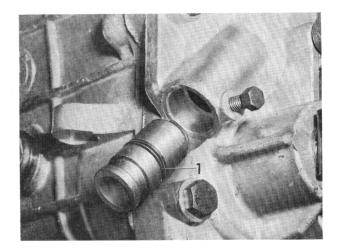
In the case of oil loss through the sealing ring (1) the plug-in bush must be renewed.
