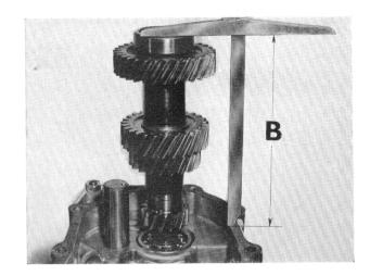
Determine thickness of shim C.
