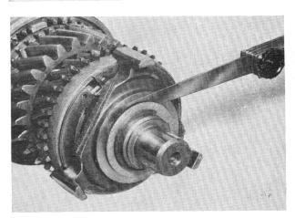
Press out the output shaft.
