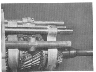
Fit selector rod of 3rd/4th gear.
