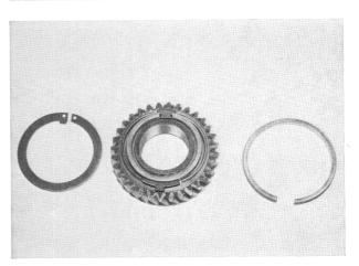
Push synchromesh ring into selector sleeve. Front edge of selector sleeve and synchromesh ring must be in the same plane.
