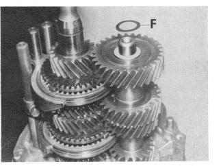
Determine thickness of shim F and place on layshaft.
