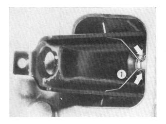
Replace lubricating felt pad in the knuckle bolt if it has become loose or dry.
