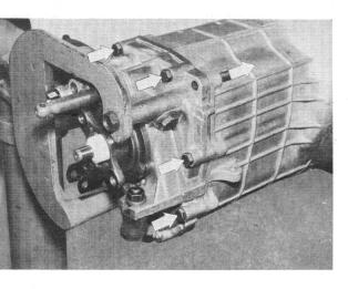
Unscrew fixing bolts on gearbox housing cover. Drive cylindrical pins out of gearbox housing.
