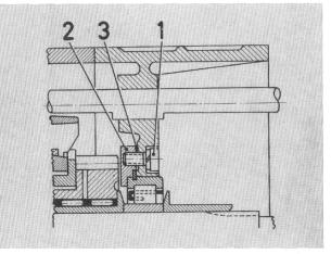
Unscrew socket head screws (1) and remove retaining keys (2).
