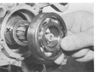
Place the previously determined shim X in front of the speedometer pinion.
