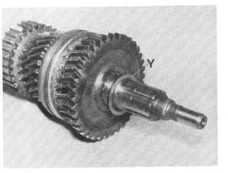
When installing: Install the 3rd/4th gear sliding sleeve with the groove in the sleeve facing the 3rd gear pinion.
