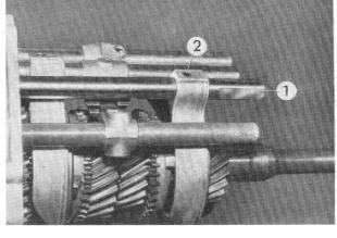
Withdraw selector shaft (3) forwards; for this purpose swing selector bar upwards.
