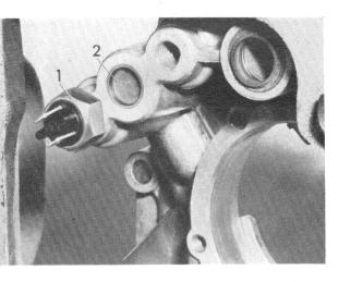
Remove reversing light switch (1) and sealing cap (2). The arrestor balls should be pushed down with a screwdriver through the exposed bores.
