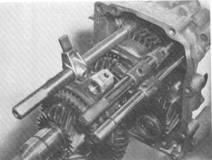
Push selector fork of 3rd/4th gear into selector sleeve. Fit selector shaft.
