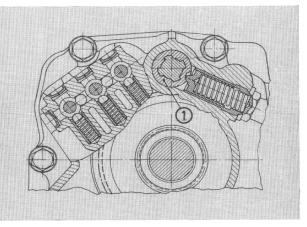
Fit wedged bush (1) in correct position. Insert clamping and locking balls through the open drillways. Using a screwdriver, push clamping balls down. Then fit shifting rods in position.
