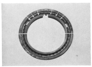
After assembly it should be possible to turn the synchromesh ring easily by hand.
