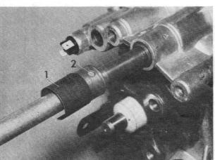
Push back spring sleeve (1) and drive out cylindrical pin (2). Pull off selector shaft and joint.
