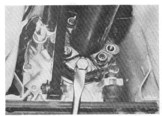
**Fitting instruction:** Do not damage screw thread. Push 'Guibo' coupling upwards as necessary. Only use lock nuts once.
