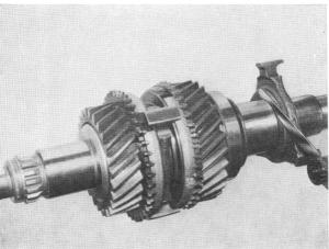
Fitting instruction: Shim up individual parts at shaft section X with shim (A) to 0-0.09 mm (0.0.0035").
