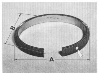
Press the synchromesh ring into the selector sleeve. The front faces of the selector sleeve/synchromesh ring must be level. The synchromesh ring must be renewed if both ends have spread excessively.
