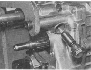
Remove locking pin in neutral position.
