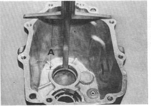
Before continuing with assembly, check layshaft, install and fit.
