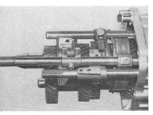
Screw gearbox cover intermediate housing with the help of two bolts. Press the shift rod for the first gear and the reverse gear into idling position.
