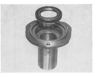
Renew radial seal in the guide sleeve — open side faces gearbox housing.
