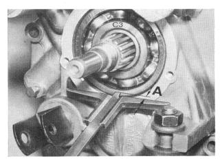
Determine distance B with seal in position, e.g.  $2.8 \text{ mm} (0.11^{\circ})$ .
