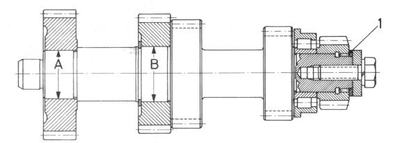
Press roller bearing of output and layshaft into intermediate housing.
