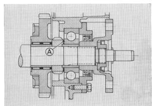
To make sure that gear mesh is correct, measure distance (C) from the cover sealing surface to the speedometer drive wheel. This shoul be 22  $\pm$  0.1 mm (0.8661  $\pm$  0.00394").
