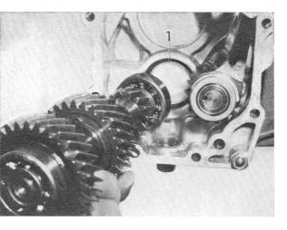
Drive layshaft out forwards with plastic hammer. **Warning:** Shims (1).
