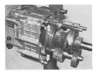
Pull gear assembly with intermediate housing, selector shaft and selector rod of 1st/reverse gear from gearbox cover.
