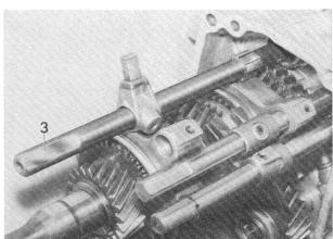
Set selector sleeve to neutral position. Remove selector fork.
