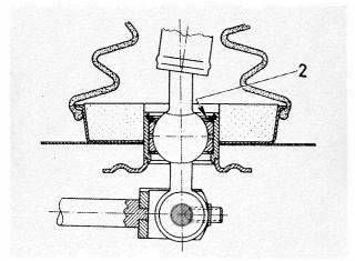
Fitting instruction: Insert ball cups with Longterm 2. Refit gear lever with shims (2) to obtain tight fit.
