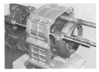
Fit reserve gear onto output drive shaft.
