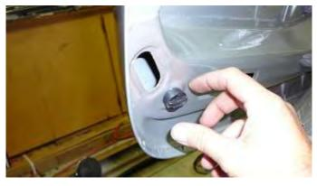
Finally, the two vibration dampeners are installed in the front. These screw in or out for adjustment. These can lift the front corners of the hood slightly and improve the front hood gap.
