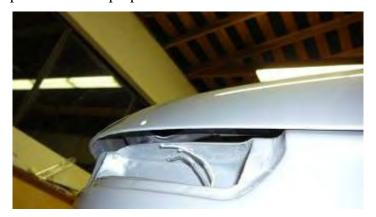
Re-install the front signal lamps and close the hood and verify clearance. If the hood is too tight at the ends and touches these, you can adjust it up by screwing out the bump stops. This probably only applies to NA cars that use the bigger lamps.
