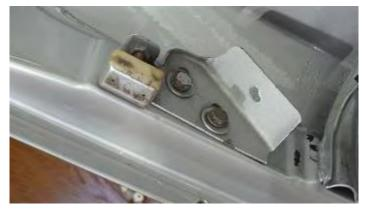
Remove the angle brackets so they will not interfere with the next adjustments.
