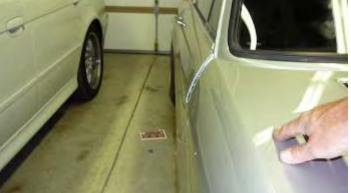
Another way to verify the correct height is to look at the car from the side, the holes for the aluminum trim on the hood should line with those on the door.
