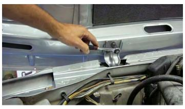
Secure both torsion arms to the apron brackets. Slide the arms all the way to the front. Make sure that your washers are positioned such that the attaching point allows the arm to rotate freely. CAUTION: do not ever attempt to close the hood with these loose, make sure they are tight on the apron slides - otherwise, you will end up with some nice scratches on your apron.
