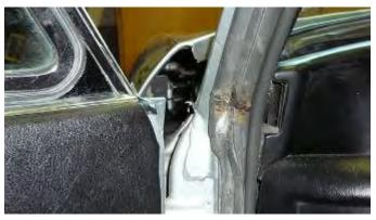
The next step is to position the keepers on the side of the apron. This is accomplished by bringing them outboard and finger tightening both screws. As you close the hood, it will position them in the correct place. Repeat this step and peek with the door open, to make sure they just touch the sides of the stoppers. The keepers can also be used to push the side of the hood outboard in order to make them flush with the side of the door.
