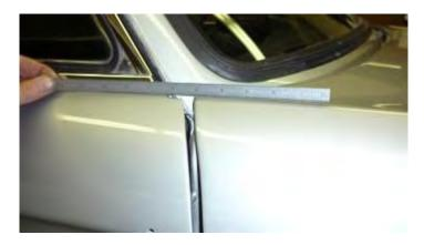
The reason for that is because the sides of the hood are angled, an incorrect height will appear to bring the sides of the hood in or out relative to the sides of the doors. The next figures illustrate:
