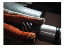
7. Remove helical gear, trust washer(S) and fiber washer (make note of trust washers stack up)
