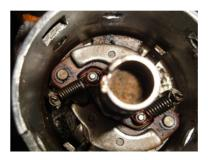
5. Remove cam upward. There should one trust washer under cam. Note a washer and O-ring clip under top felt pad
