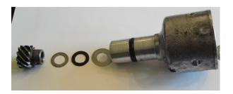
8. Pull out shaft with counter weights. Again make note of trust washer(s) and fiber washer located underneath counter weight shaft plate. On mine fiber washer was absent under main plate, which explained excess axial play.
