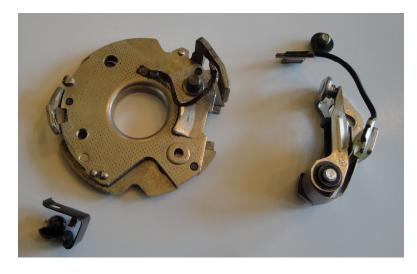
16. Set contact breaker to specs, install the distributor and last set engine timing
