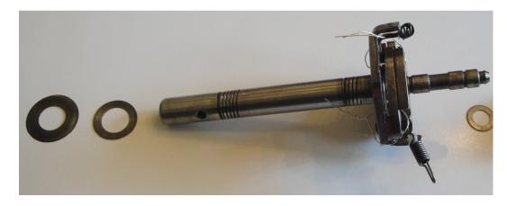
9. Clean all the parts with your favorite cleaner. Remember to take a lot of pictures at each disassembly stages. Measure trust washer(s) and fiber washer for each group and make notes.
