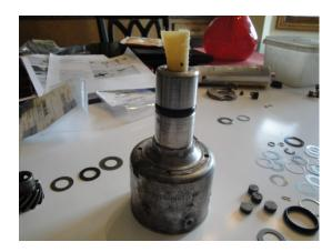
13. Lubricate shaft assembly, counter weights, springs and with predetermined trust washer and fiber ring sizes slide shaft assembly onto the housing. Slide cam with trust washer over shaft and then secure cam with washer and ring.
