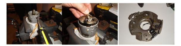
4. Disengage two springs from cam base posts and rotate springs outward. Force cam upward with two screwdriver until retaining clip is out of groove (do not remove felt inside cam before cam disengagement)
