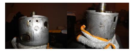
3. From vacuum regulator opening, insert screw driver and pry contact breaker plate up at each indent locations.
