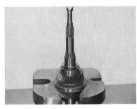
Fitted position of individual parts: Spacer bush (1), shim (2), roller bearing (3), spacer bush (4), needle bearing (5), 2nd gear pinion (6), selector sleeve (8), 3rd gear pinion (9) and needle bearing (10). Fitting instruction: Check synchromesh units; see page 23—00/29.
