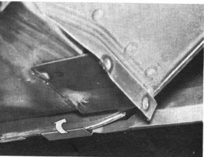
Bend over edges of the panel after fixing the side panel.
