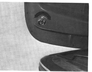
The lid will make good contact if the rubber buffer stops at the front are adjusted; these can be set higher or lower by turning.
