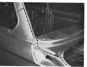
Separate roof pillar at the rear swaged edge and past the ventilation opening as far as the luggage compartment cutout.
