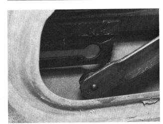
Loosen the glass holder retaining bolt. Take out the glass holder and the stop angle.
