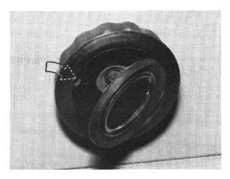
Loosen and remove screw (6). Take off the handwheel (7) and bezel (8).
