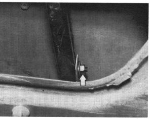
Detach the lower rear window guide rail and remove.
