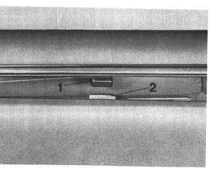
The rubber buffer stops (1) must be adjusted to touch the retaining angle pieces (2) and therefore prevent the lid from vibrating.
