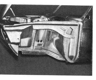
Apply Terostat tape. Fit side panel.
