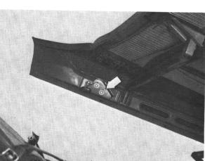
The gap is adjusted by sliding the angled catch to the left or right.
