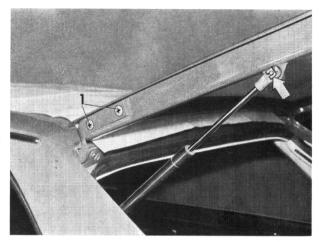
Adjust the rear door panel so that the side pillars and tail panel edges are aligned with the door.
