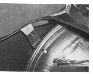
Separate the side panel from the body tail panel and also from the base of the luggage compartment along the line of spot welds.
