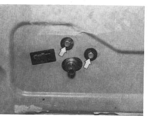
Remove remote door operating mechanism.
