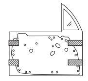
7. With masking tape secure the liner in place until set.
