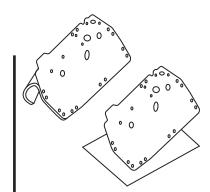
5. Start by partially detaching the up side of the liner from the back paper. Match the perforations and the gaps of the door. Once in place pull down the backing paper completely against door while doing it.
