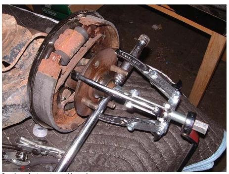
**Sneak peak at next month's work:** There was one right rear hub really frozen to the stub axle. I'm quite sure it hasn't been off the car since 1974. The two have been separated now from birth with the help of a wheel puller and an 8 lb sledge hammer. These will be powder coated and new hardened wheel studs installed. TII NOTE: Little known fact, but these rear hubs is an NLA part, they are hardened on TIIs to be stronger. A part worth obtaining for other upgraded 02's if you find a parts car.
