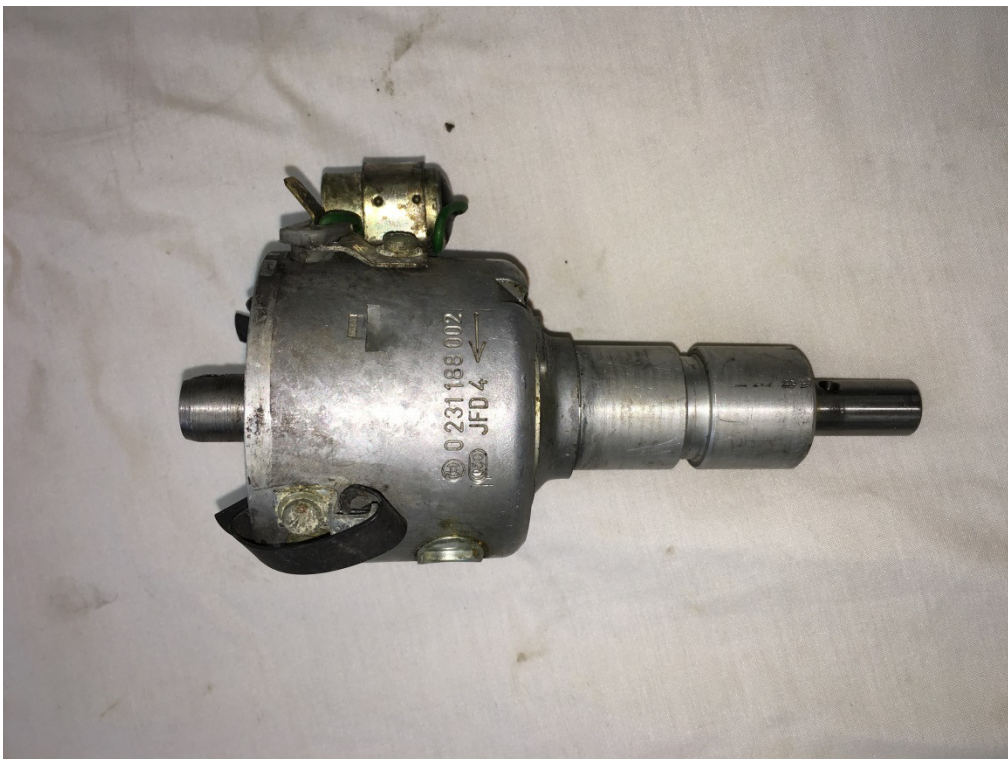
Mechanical advance distributor Missing the gear on bottom of shaft $50
