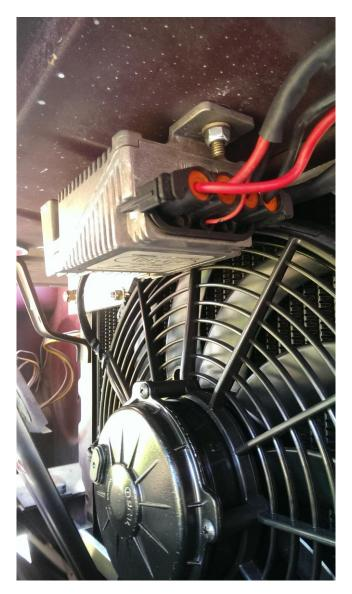
These modules have an interesting PWM input requirement, as the table below shows. Between an input of 10% and 90% duty cycle, the output varies linearly.
