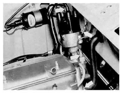
Removal of upper timing case cover - 11 14 100. Move cylinder in piston 1 to TDC.
