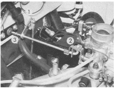
Loosen clamp screw (1) in clamp (2). Pull out choke cable. **Fitting instruction:** Secure choke cable sleeve. **Warning:** Sleeve may project forwards by 15 mm (0.59") max. otherwise the choke flap will not close fully. Push choke cable at instruments panel into the bottom notch. Press choke lever (3) against stop. Tighten clamp screw in this position.
