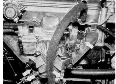
Pull fuel hose off fuel pump and cable off remote thermometer switch. Remove water hoses from branch stub.
