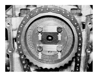
**Note when fitting:** Fit chain in such a way that the hole for the dowel pin faces downwards. The notch in the camshaft flange must be aligned with the cast projection in the cylinder head.
