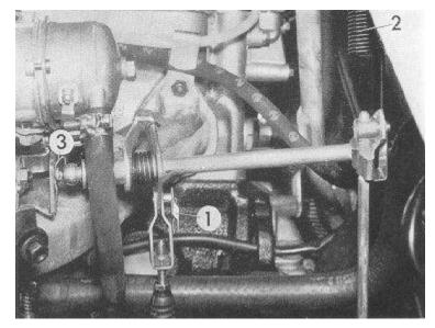
Remove vacuum hose with check valve from threaded manifold and detach warm water hoses<sup>1</sup>) form intake manifold. Remove oil dipstick holder.
