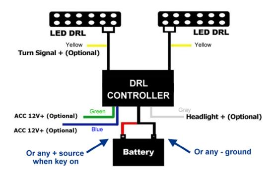
When yellow wires are connected to turn signals, DRL lights flash with turn signals.
