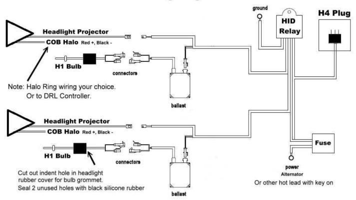
**NOTE:** Black and blue wires with red insulators and a male connector with yellow weatherproof gasket should be cut from light blue rubber grommet and discarded as they are not used in this installation. Our HID controller will make the needed connections.
