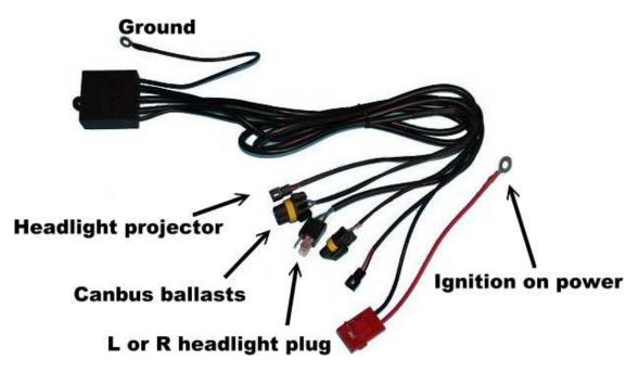
Note: For this HID conversion installation, the (blue & black) wires shown below and ballast plug that are included in the ballasts & bulbs box are not used. They may be cut and discarded. Only the (orange bulb connector) to ballasts are used. Your kit wires may have already cut.
