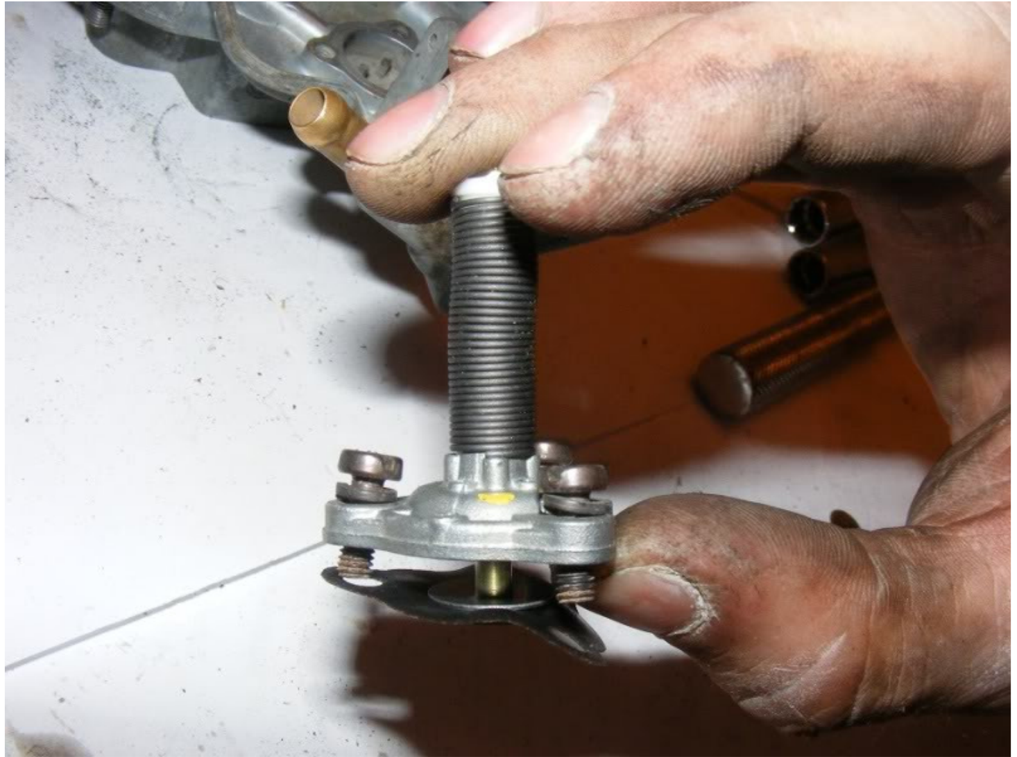
Step 107 - Tighten the 3 screws evenly and check operation as per step 25
