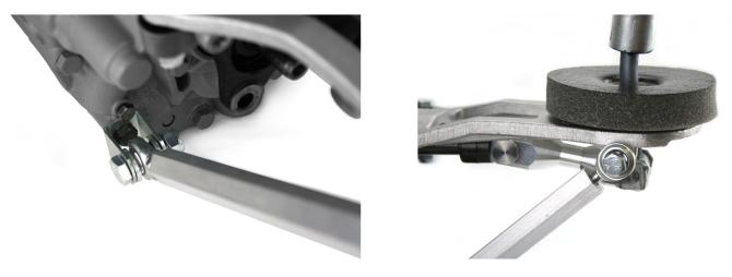
Attach transmission mount to rear support bracket and attach to transmission as shown.
