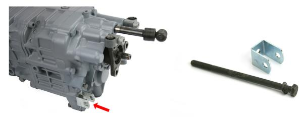
Attach locking end of adjustment bar to lower support bracket using included hardware. Spacing washers should be used on both sides of the ball joint. Attach other end of support rod to shifter platform using supplied bolt and thread locker compound. The hex support rod can be turned to adjust height angle of the shift platform as necessary. Once any necessary adjustments are made, tighten lower securing nut to lock the support rod length in place.
