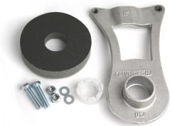
From inside the vehicle cabin, install the shift cup bushing onto shift lever, then into the shift platform. The shift bushing has two tabs that index two slots in the shift platform. From under the vehicle, attach the DSSR to the shift lever. If you're using a late 4-spd shift lever, you'll need to use the included yellow shim washers for proper fitment. If you're using a Z3/Z4 shift lever, the included washers are not necessary. Install pins and retention clips to DSSR.
