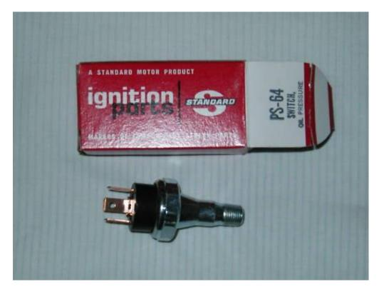
The switch will also let the pump run when you hit the starter because the engine doesn't have oil pressure yet.
