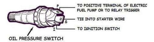
One wire goes to the pump, one to the start circuit, and the other to the ignition circuit. So, when there is no oil pressure, the switch connects START to PUMP, and as soon as you start cranking it runs the pump. When the oil pressure comes up, the switch connects IGN to PUMP, for normal running. When oil pressure goes away (because you just hit that rock and tore the pan off the engine, for example) it again connects START to PUMP, and disconnects IGN from PUMP, so the pump shuts off.
