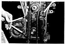
20. Replace the timing chain guide and tension rails as shown.
