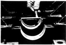
11. With the engine block upside down, install the remaining bearing shells in all the main bearing caps and saddles, making sure everything is clean and dry.
