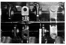
32. Place oil sprayer bar into position, then turn upside down to:
