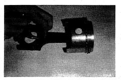
9. Likewise assemble a connecting rod (dry), complete with bearing shells and measure the shell inner diameter, the rod journal size and take their difference to find the clearance. Again, verify that these clearances conform to specs.
