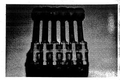
2. Before removing any other pistons, use your number punch to mark one side of the big end of the rod. Stamp both the rod and its cap with the number of the cylinder [numbered from the front of the engine]. Repeat this procedure for all the rods of the engine.
