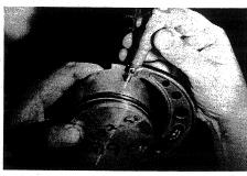
${\bf 2}.$  Use mic to measure piston diameter (perpendicular to wrist pin).
