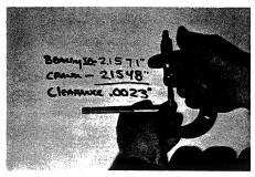
8. The difference in the two measurements will represent the bearing clearance and it should meet factory specs (the general rule of thumb is .001" clearance for every 1" of journal diameter).
