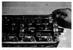
31. When all head bolt slots align with all bolt holes, insert one bolt for each of four shafts to anchor shafts.
