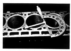
1. Remeasure cylinder bores with snap-gauge and  $3^{\prime\prime}\text{-}4^{\prime\prime}$  micrometer.
