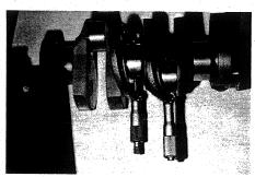
4. Use your 2"-3" mic to measure all of the main bearing journals, and the 1"-2" one for measuring the rod journals. Whether standard or ground undersized, compare measurements with factory specs to verify all are within tolerances (some machine shops purposely grind for extra clearance to "cover" themselves).
