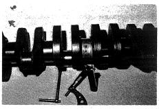
5. Place the middle (thrust) main bearing on the center main journal and use a feeler gauge to measure the distance between the side of the bearing and the crank.
