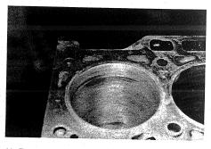
11. The first few passes will dress most of the cylinder wall with exception of the typical low spots at the top and (frequently) the bottom of the piston rings' travel. It is not necessary to completely remove thes low spots, but only to prevent them from totally encircling the cylinder (as shown). Also ideal cross-hatching at between 45 and 60 degrees from horizontal.
