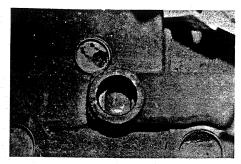
16. Enlarge the inner port of the plug hole at the back of the coolant galley with your die grinder. Increase the size of this hole by about 50% to 75% to force more water circulation to the center and back of the engine block.
