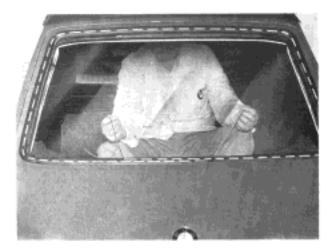
Fit the filler strip into the rubber surround. Seal the glass with Teroson Sealing Compound 2322.
