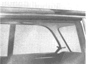
When correctly adjusted the window must locate neatly at the top on the rubber seal.
