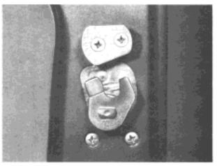
Loosen screws for toggle spring lock.
