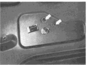
Detach connecting rod of remote control mechanism.
