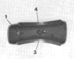
Unscrew nuts (1 and 2) and remove rubber pad. Installation instructions: Ensure correct seating of underlay (3 and 4).
