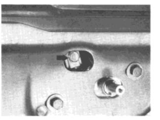
Slacken retaining screw on worm gear.
