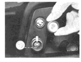
Unscrew the knob from windshield wiper switch. Unscrew bezel and withdraw the switch to the rear. The cables remain connected. Remove the cable from the cigarette lighter.
