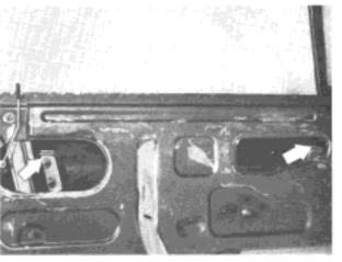
Adjust the two stops so that they locate on the welded angles when the window is wound up.
