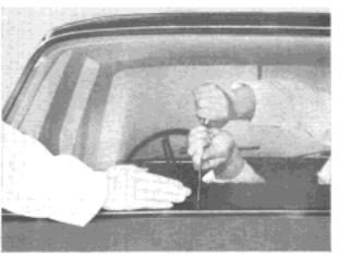
Place preassembled windshield on windshield aperture and hold firmly to prevent slipping to one side. Pull rubber seal over body web using string. During the fitting procedure use suitable pad or flat of the hand to bring windshield into correct position by knocking in regular pattern.
