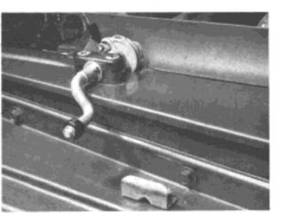
Loosen wire cable at clamp disc.
