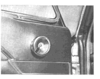
Loosen screw and remove handwheel.
