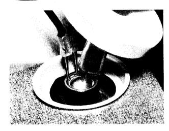
Fitting instruction: The thickness of shim (A) must be chosen so that the selector lever can be moved easily without play.
