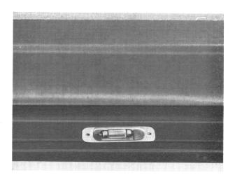
Press bulb out of holder and remove.
