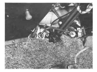
Pull out speedometer shaft together with rubber sleeve. **Note when fitting:** Note correct length of speedometer shaft 1).
