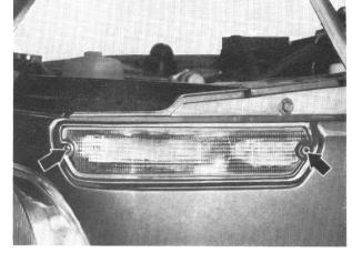
$\label{lem:decomposition} \mbox{Disconnect cable and remove bulb holder with lens.}$
