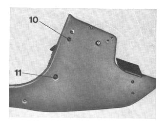
Locate the fixing holes (10 and 11) on the left and right side panels and pierce the facia.
