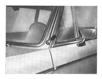
Slide the antenna through the antenna supports and screw on to the base.
