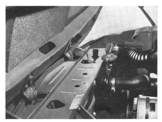
Connect earth (ground) cable from right hand hinge on the bonnet (hood) to the body.
