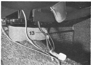
Connect the battery cable to the existing plug (13) on the wiring for the hazard warning flasher switch.
