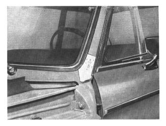
Drill fixing holes for the base of the antenna.
