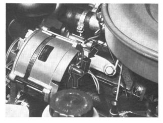
Connect the suppressor condensor to the alternator terminal B  $\,\pm\,.$
