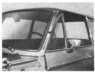
Push antenna cable through the slot in the window member into the inside of the vehicle.
