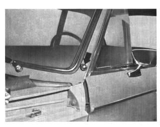
Undo screws (1 - 4) and remove the lower left hand facia trim.
