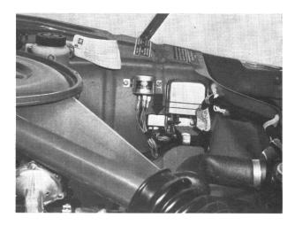
Connect the suppressor condensor to the regulator.
