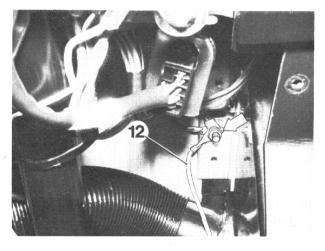
Attach the earth (ground) cable (12) to the heater fixing screw.
