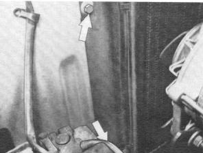
If radiator is fitted with oil cooler, detach inflow and reflow pipes.
